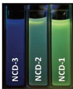
Figure 1. Optical images of different samples in distilled water under 365 nm UV light.
