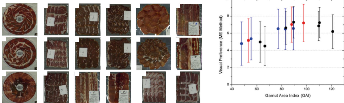
Fig. 1. Left: The 18 sausage samples used in the visual experiment (D65 illuminant). Right: Average visual preferences and standard deviations (magnitude estimation method) for 20 Spanish observers vs. values of Gamut Area Index [2] (results for 3 CIE standard illuminants, 5 CIE Blue LEDs and 7 light sources in red, blue and black colors, respectively).
