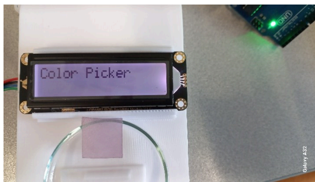
Fig. 6. Color Picker system showing the color of the plasmonic paper on the display.
